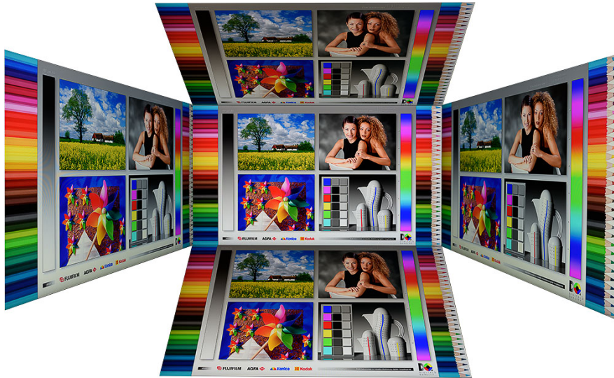
Horizontal and vertical viewing angles
